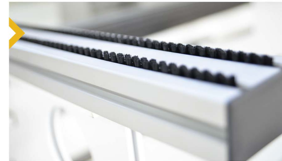
Front support arms with brushes are mounted on a linear guide rail system
